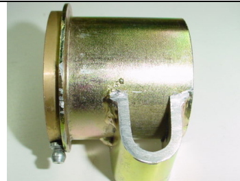
Bushing installed in provided rear control arm mount
